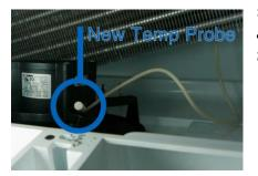
tape and attach to the fan unit.
